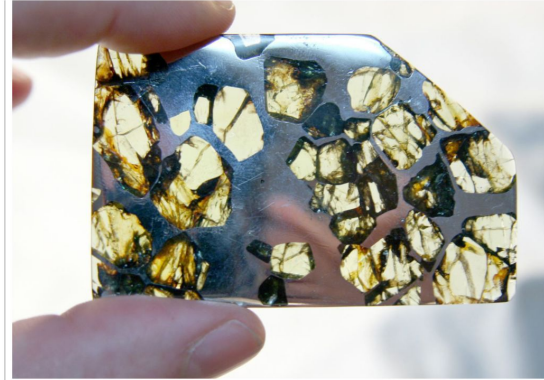
A slice of the Equeul meteorite. This type of meteorite is from the core-mantle boundary of an ancient planetoid that was smashed apart billions of years ago. DOUG BOUMANN
