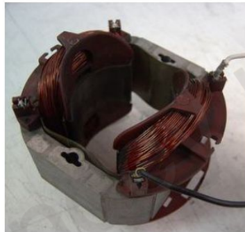
The stator of a vacuum cleaner showing two electromagnets. MARRRCI (CC BY-SA 3.0)
