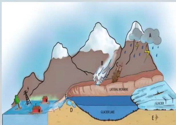
Figure-1: Illustrative graphic showing various reasons for GLOF occurrence (A) Cloudburst (B) Snow avalanche (C) Landslide (D) Melting of ice in moraine (E) Earthquake (F) Overflow
